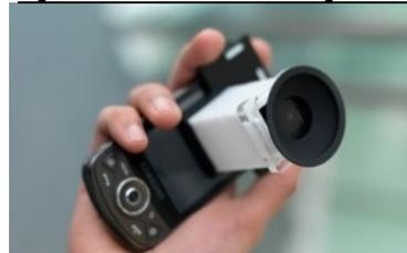
The Netra is an inexpensive clip-on eyepiece that goes on top of a cell phone. The user looks through this eye piece and interactively aligns the displayed patterns by clicking the buttons. The number of clicks required to bring the patterns into alignment indicates the refractive error. The device is not available commercially yet and is currently being optimized with eye care professionals. However, its target market is the developing world where the need is great.
